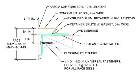
PRE-DRILL WITH 3/16-IN. DRILL BIT FOR MASONRY CONDITIONS.
